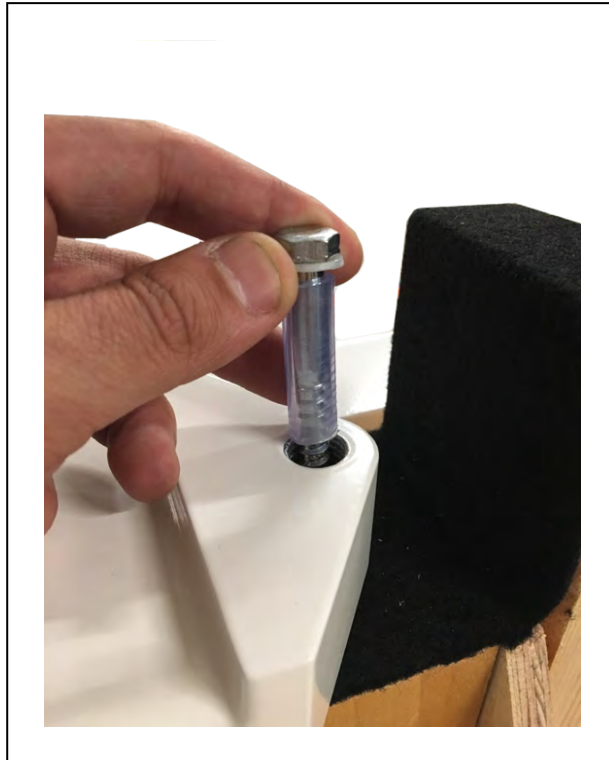
Figure 9-3. Removal of Bolt
