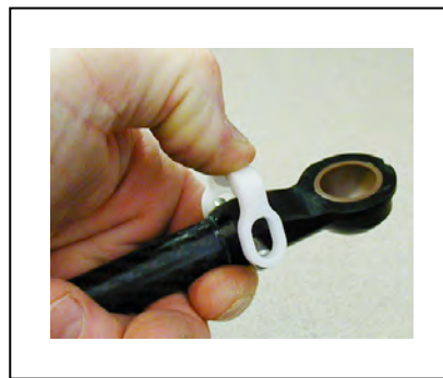
Figure 6-13. Push the retainer Into Position
