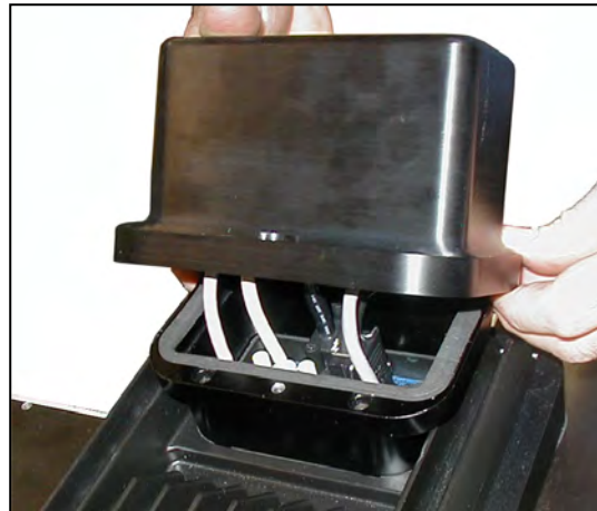
Figure 4-23. Installing Cable Entry Top Cover Assembly
